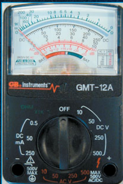
6. Here is a standard, four function analogue multimeter.
